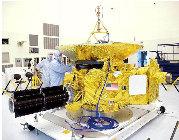
New Horizon Space Probe, in assembly before launch. The black tube is the thermoelectric-radioisotope generator. NASA
