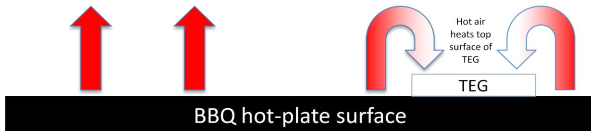
To counter this possibility, all the following TEG experiments incorporated a fan blowing over the top of the experiment to try to stop convection currents. This seemed to help, because later measurements showed more of a temperature difference between the top of the TEG and the BBQ or frypan surface.
