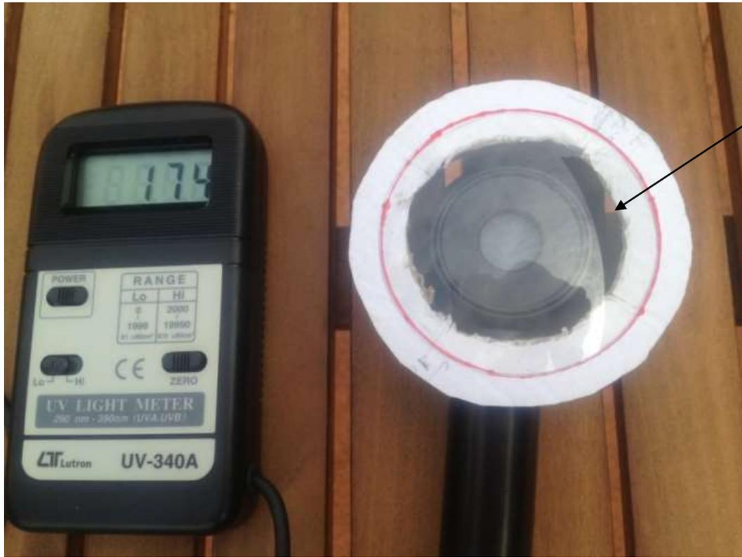
The glass lens was placed on top of the platform, and aligned with the circle marked in red pen. This was exposed to the UV rays of the sun for five seconds, before recording the measurement.
