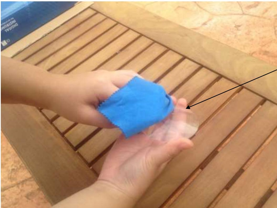
Lens was cleaned with the microfiber lens wiping cloth by holding the lens by the rim, to remove any dust and fingerprints which may block UV rays
