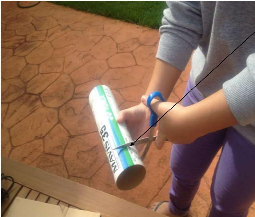
The cylindrical cardboard tube was cut so the height is fractionally higher than the sensor.
