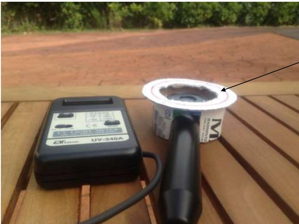
The UV detector was placed directly underneath the platform and measured the amount of UV rays without any lenses, as the control.
